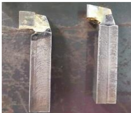
Fig. 4. ISO 6 chisel with a carbide bit.
