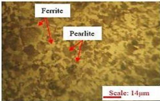
Fig. 4. Micro-structure of S45C non-treatment
