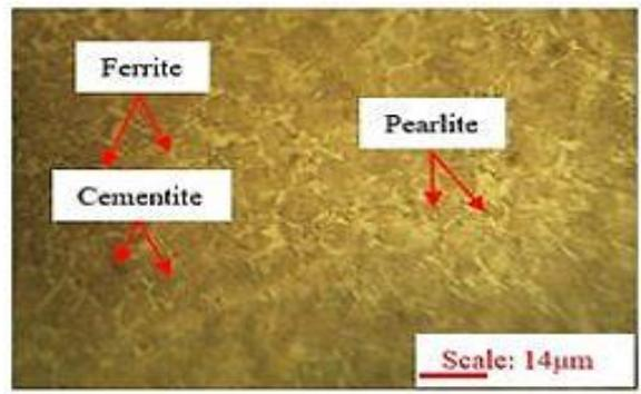
Fig. 7. Micro-structure of S45C quenched in oil
