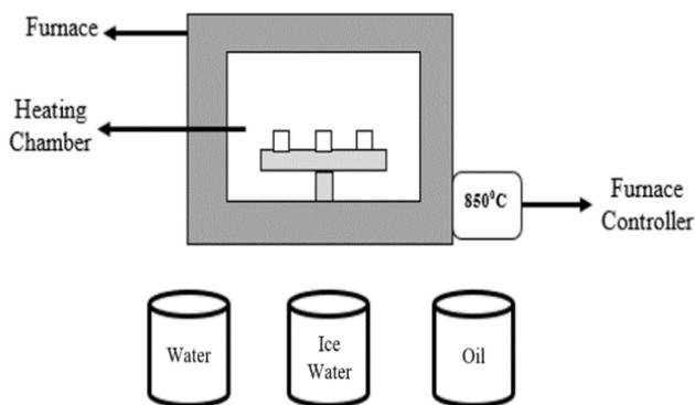
Fig. 2. Cooling fluids in heat treatment processes
