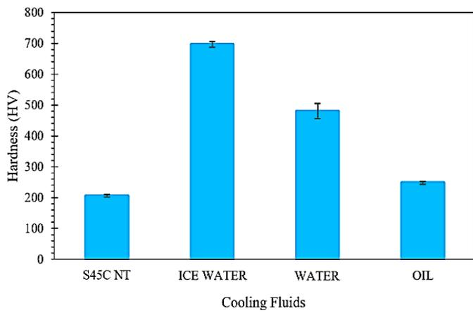
Fig. 3. Hardness values before and after heat treatment process with different cooling fluids at S45C
