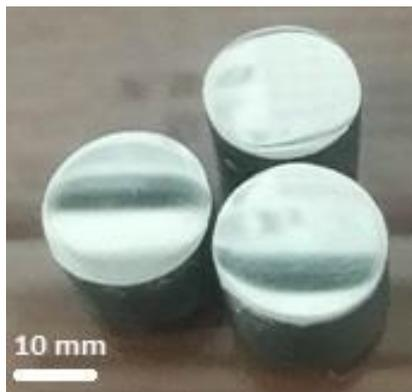
Fig. 1. S45C carbon steel specimens
