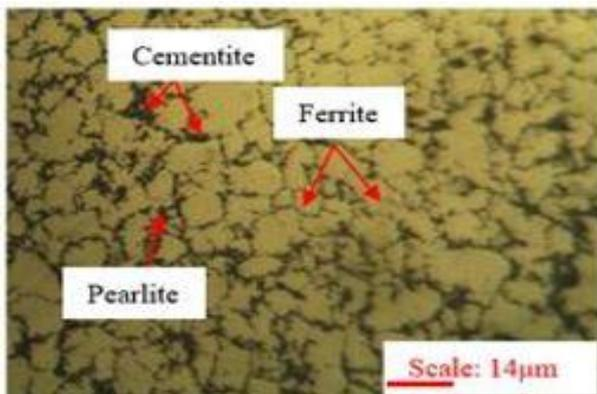
Fig. 6. Micro-structure of S45C quenched in water
