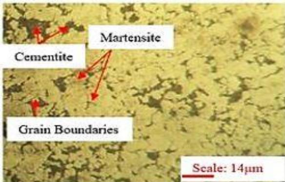
Fig. 5. Micro-structure of S45C quenched in ice-water
