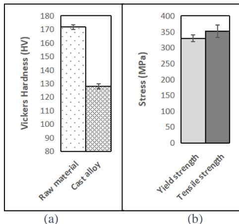
Fig. 5. (a) Vickers hardness, and (b) Tensile strength of the Cu-Zn alloy.
