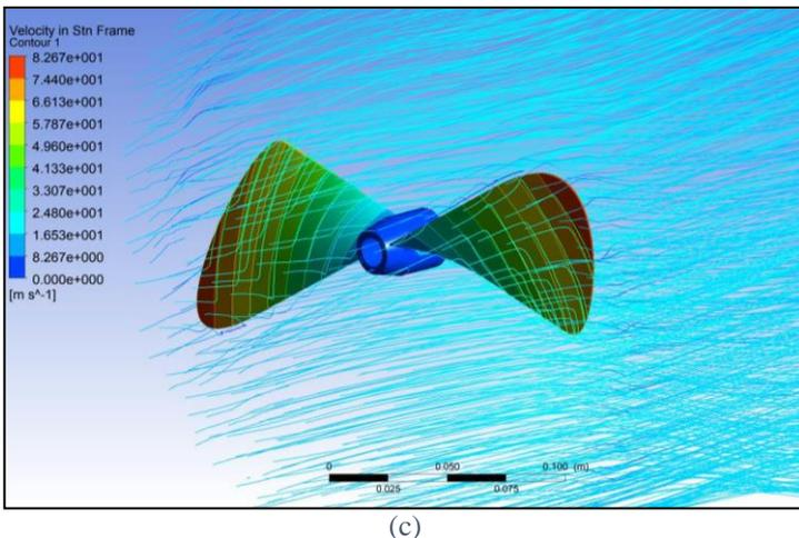
Fig. 3. (a) Turbulent kinetic energy, (b) density streamline characteristic, and (c) velocity distribution for the propeller.
