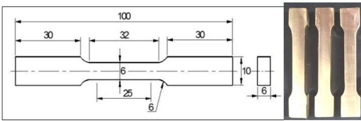
Fig. 2. ASTM E8-09 tensile test sample.
