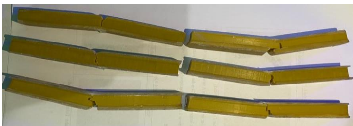
Fig. 11. Documentation of Impact Test Specimens.
