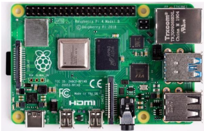
Fig. 2. Raspberry Pi 4 as the main controller
