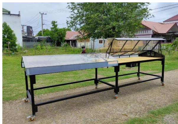
Fig. 1. Hohenheim tunnel dryer modified in Aceh.
