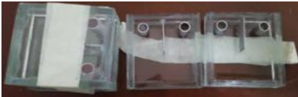
Fig. 5. Mold for crack test sample.
