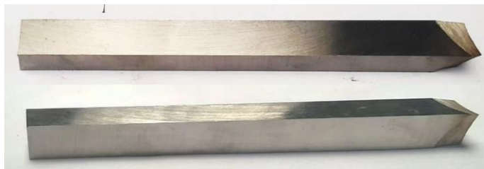
Fig. 9. The cutting tool condition before the cutting process
