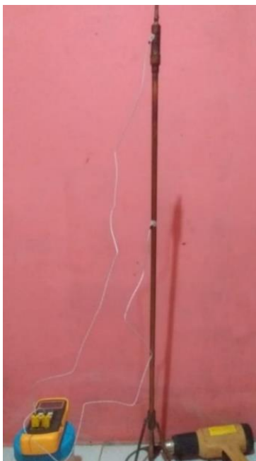
Fig. 8. The process of testing the response of the heat pipe in transferring heat
