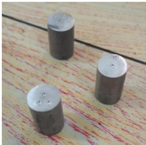
Fig. 3.Indentation marks on specimens after being hardness tested
