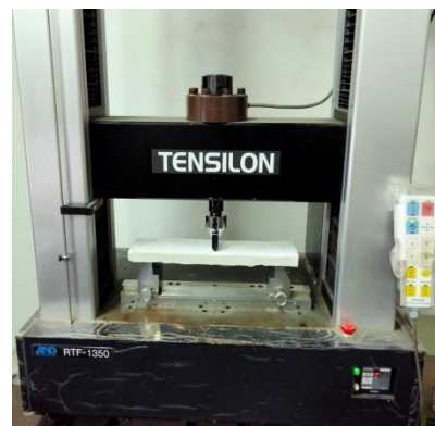
Fig. 3. Testing the flexural strength of gypsum composites
