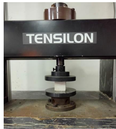
Fig. 4. Testing the compressive strength of gypsum composites
