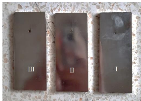
Fig. 4. Specimens after electroplating process independent of time
