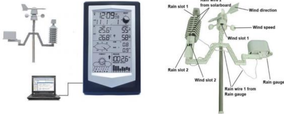
Fig. 3. Automatic Weather Station (AWS) instrumentation [10]
