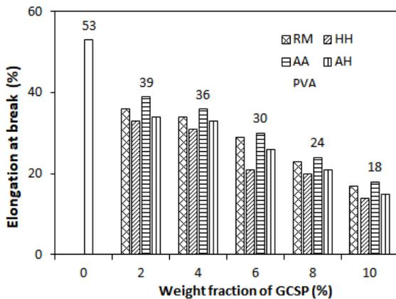
Fig. 9. The elongation at break of biodegradable film
