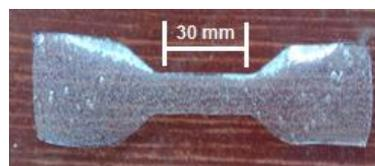
Fig. 4. Tensile test specimen of ASTM D638
