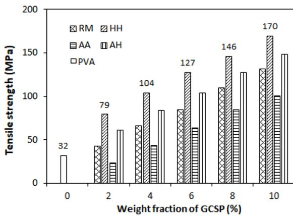
Fig. 8. The Tensile strength of biodegradable film
