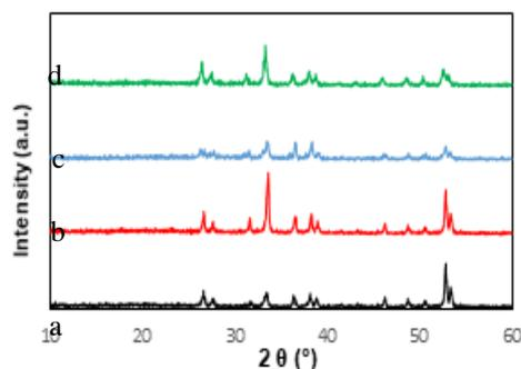
Fig. 6. The XRD patterns of a) raw GCSP; b) Calcination GCSP; c) Alkali treatment GCSP; d) Alkali treatment + Calcination GCSP.
