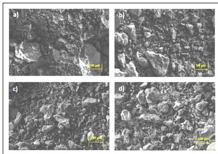
Fig. 7. Scanning electron micrographs of a) raw GCSP; b) Calcination GCSP; c) Alkali treatment GCSP; d) Alkali treatment + Calcination GCSP
