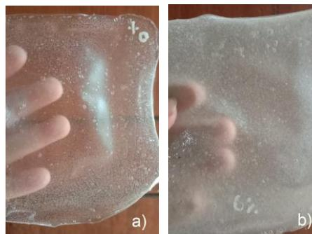
Fig. 3. Biodegradable film. a) PVA; b) PVA/GCSP
