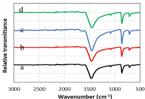
Fig. 5. The FTIR patterns of a) raw GCSP; b) Calcination GCSP; c) Alkali treatment GCSP; d) Alkali treatment + Calcination GCSP
