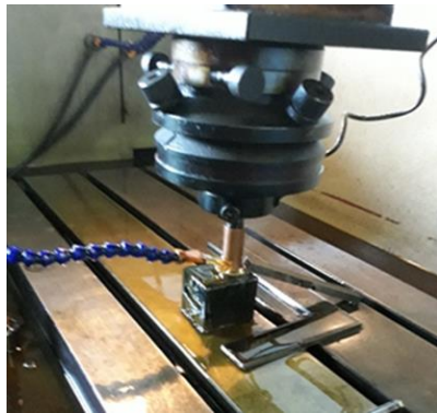
Fig. 1. Process of S-EDM with copper electrodes.
