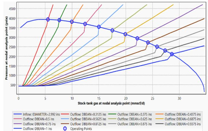
Fig. 8. Graph of operational points at tubing size 2.992" (3-1/2").
