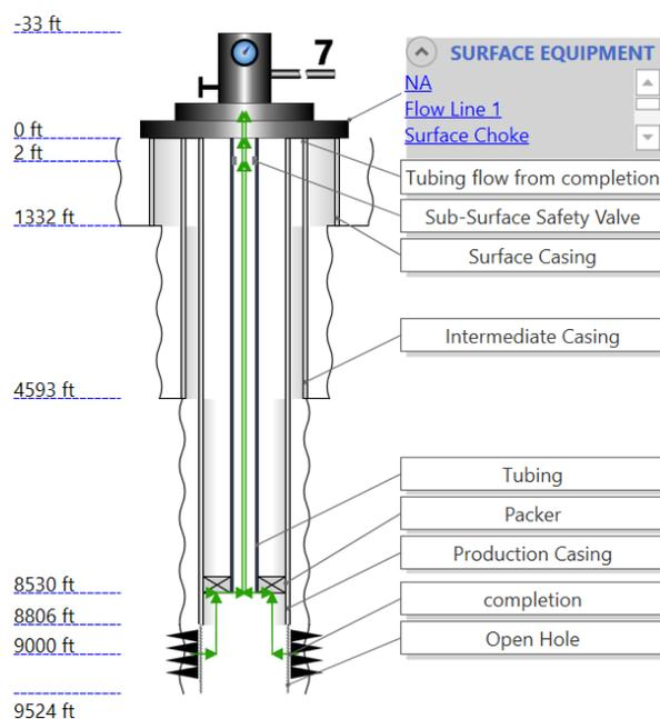
Fig. 2. Modeling of well X completion.
