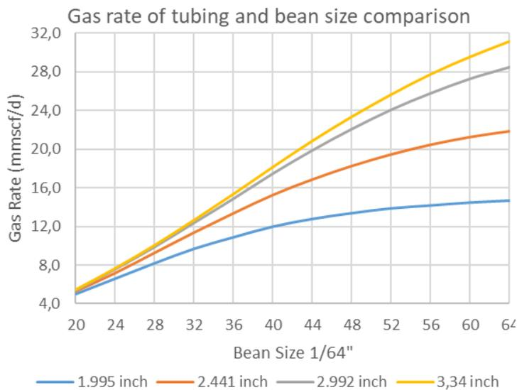
Fig. 10. Comparison of bean size and tubing size to production rate.
