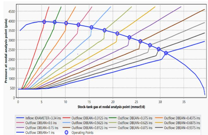
Fig. 9. Graph of operational points at tubing size 3.34" (4").
