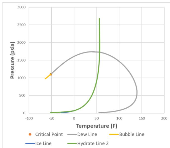
Fig. 3. Phase diagram of the reservoir fluid.
