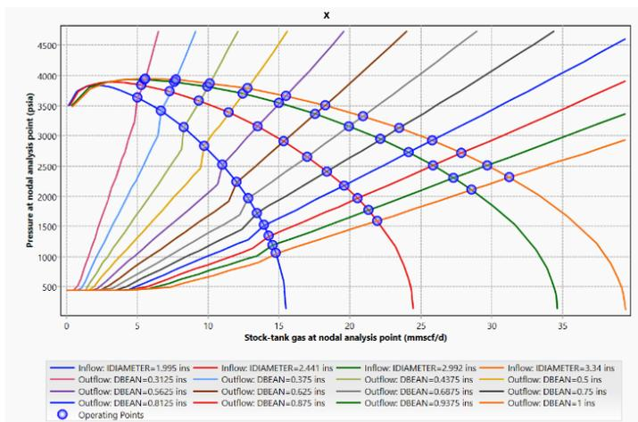
Fig. 12. Operational graph of gas production rate points with variation of tubing size and bean size of well X.
