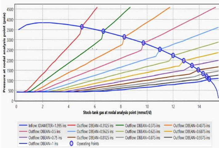
Fig. 6. Graph of operational points at tubing ID 1.995" (2-3/8").
