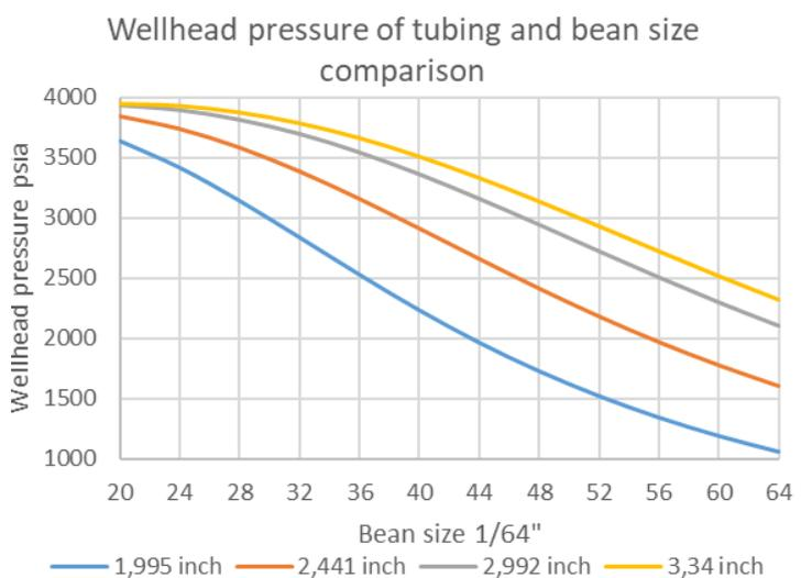
Fig. 11. Comparison of bean size and tubing size to wellhead pressure.
