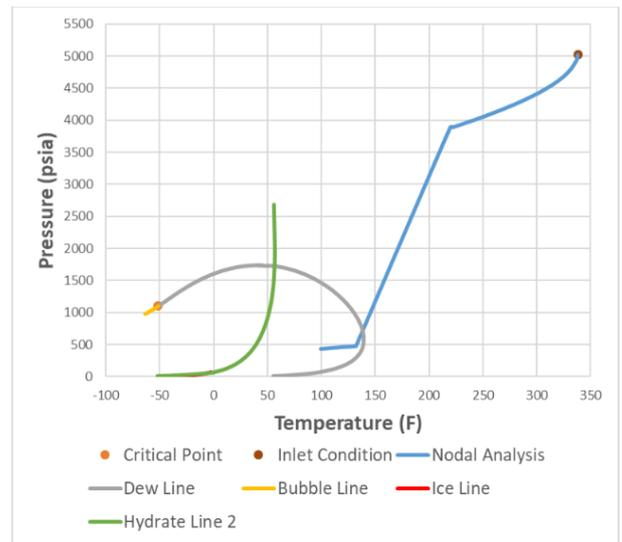
Fig. 5. Phase diagram and pressure path of the reservoir fluid.
