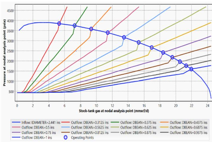
Fig. 7. Graph of operational points at tubing size 2.441" (2-7/8").
