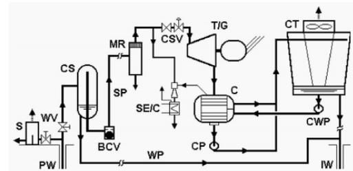
Fig 1. Simplified single-flash power plant schematic
