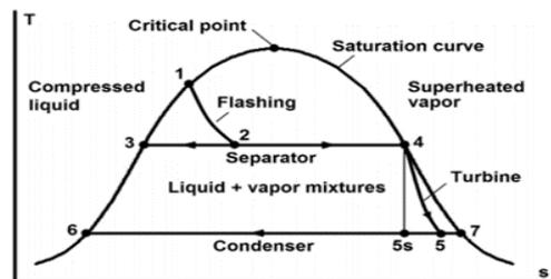
Fig 2. Diagram of Temperature-Entropy state for a single-flash plant
