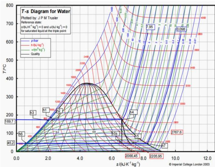
Fig 4. State point on the T-s diagram.
