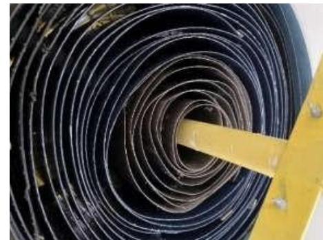
Fig. 7. Filling Material Cooling Tower
