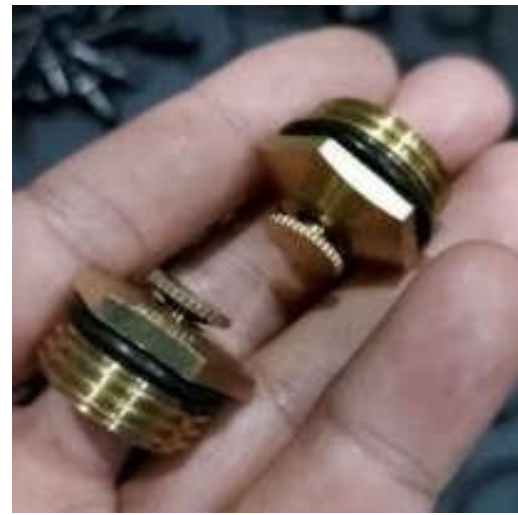
Fig. 6. Sprinkler Cooling Tower
