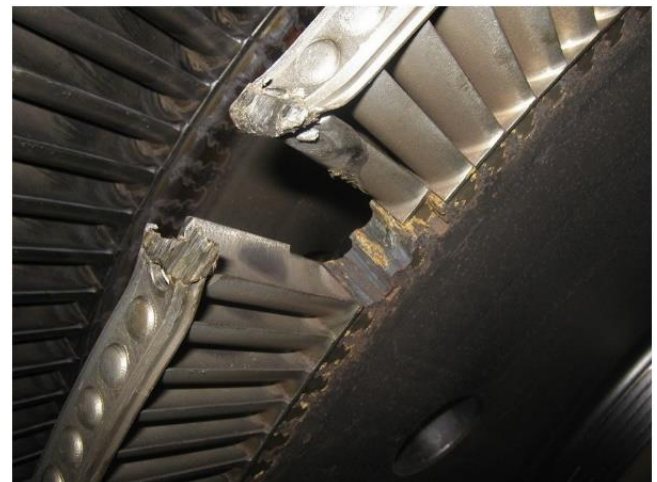
Fig. 3. Fracture surface of the rotor blade roots-5th rotor wheel [21].
