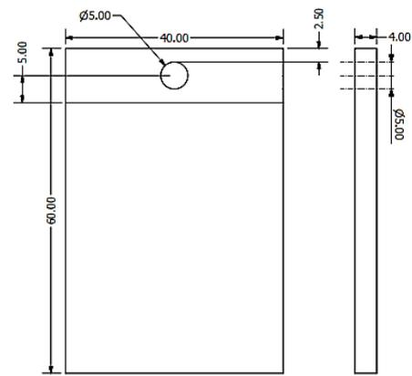
Fig. 1. Specimen size dimensions
