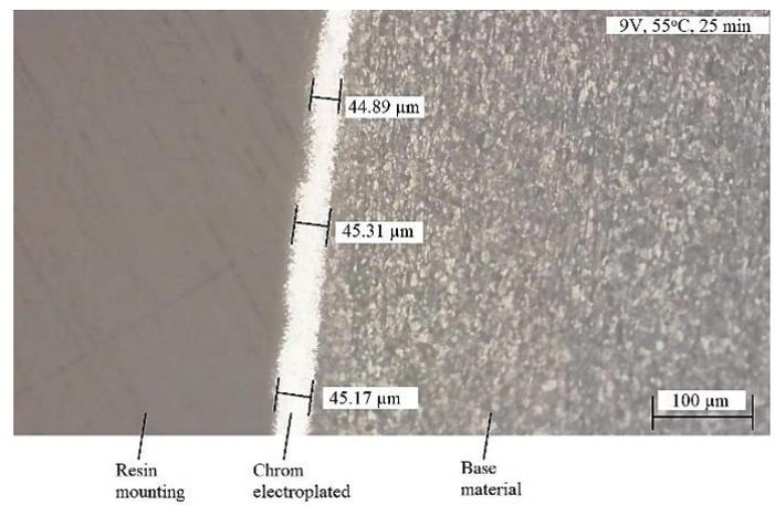
**Fig. 3.** Electroplating process result
