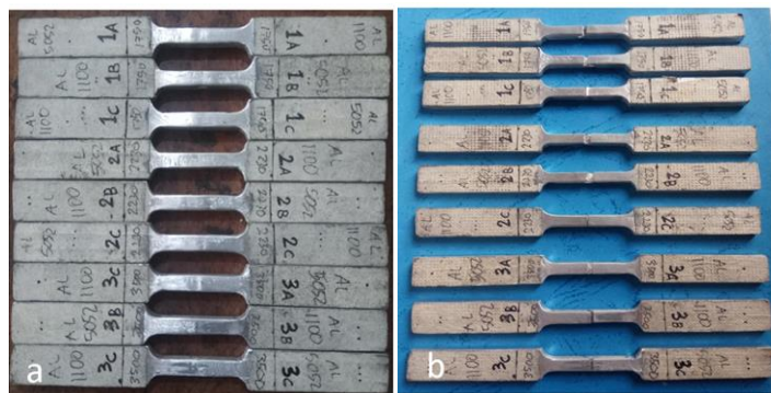
Fig. 3. Tensile test of specimen. (a) before, and (b) after
