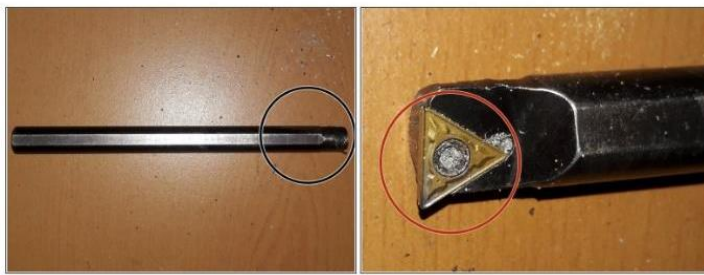
Fig. 5. Tool Condition Check
