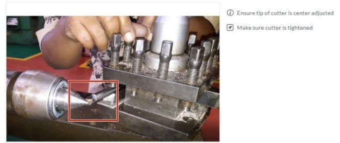
Fig. 7. Determination of Starting Point (Datum)
