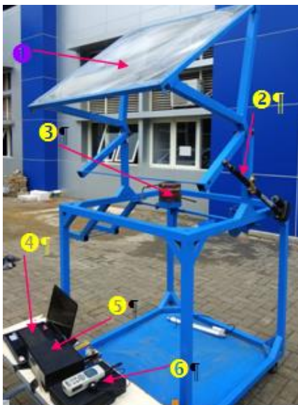
Fig 4. Photograph of experimental setup: 1–Fresnel lens; 2–hydraulic actuator for solar tracker single-axis; 3–cooking vessel (receiver); 4–Laptop; 5–Digi-Sense 12 CH-Scanning Bench top data logger; 6–SPM-1116SD solar power meter.
