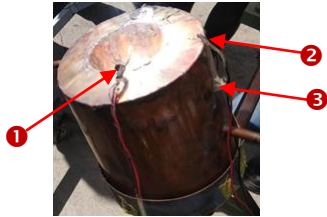
Fig 3. The position of temperature measurement by a thermocouple on the receiver: 1–focal temperature; 2–wall temperature of receiver; 3–water temperature.
