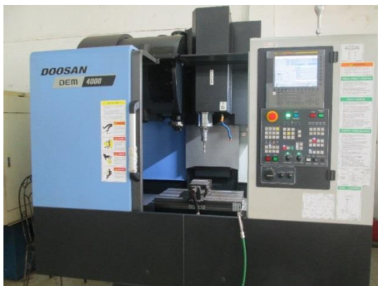
Figure 3. CNC Milling Machine Doosan DEM4000
