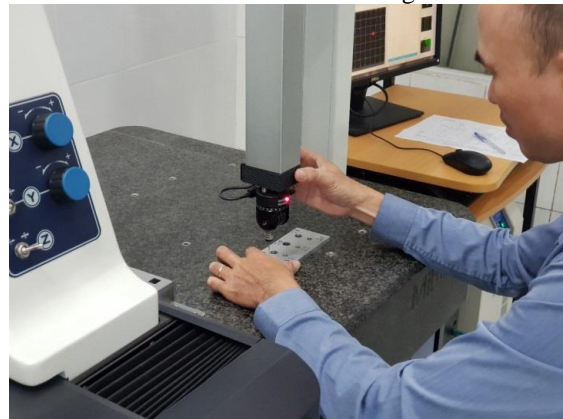
Figure 11. Measure the burr height of each borehole
