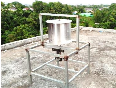
Gambar 3. Prototipe turbin angin Savonius
