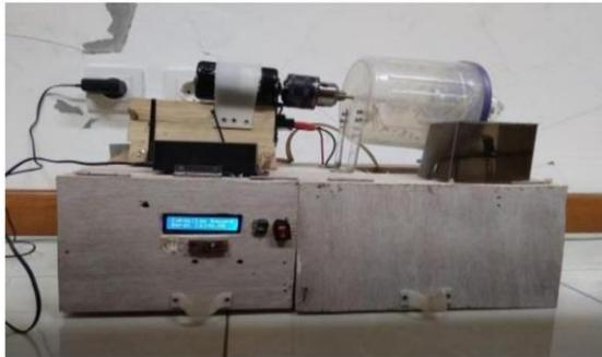
**Figure 2.** Peeler Machine Design
