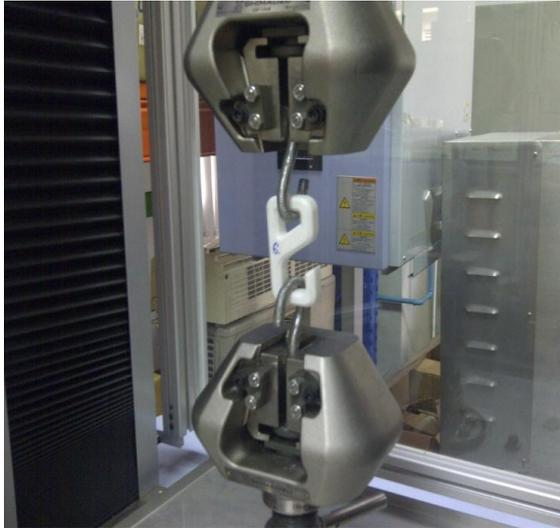
**Figure 5.** Load-bearing capacity test on SHIMADZU
