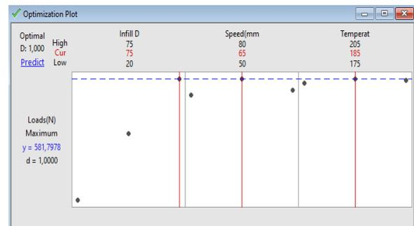
**Figure 8.** Optimum parameters for PLA-Copper material
