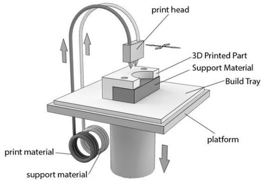
**Figure 1.** Basic FDM process
