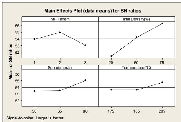
**Figure 7.** Effect of parameters on load capacity.
