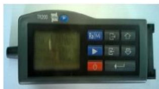
Gambar 7. Alat Surface Roughness
