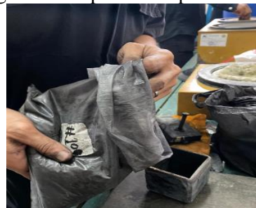
Gambar 5 Pengisian arang kedalam pack carburizing
