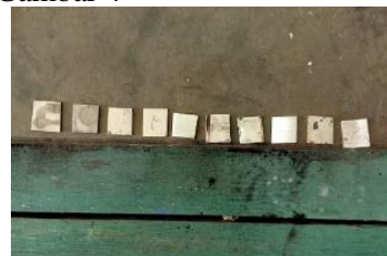
Gambar 4 Persiapan spesimen pack carburizing
