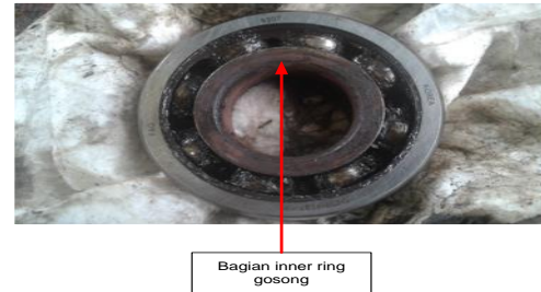
Gambar 4.9 Inner ring bearing gosong
