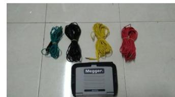
Gambar 4. Soil resistivity meter
