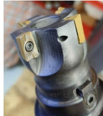
Gambar 2.2 Pahat Carbide Diameter 50 mm
