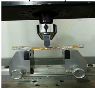
Gambar 4 Proses pengujian bending
