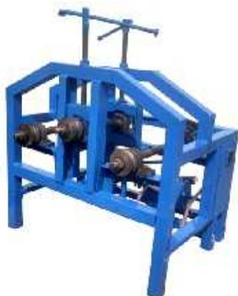
Gambar 1 Mesin Bending Pipa
