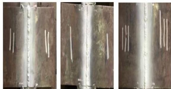
Gambar 4 Hasil Penetrant Arus 80A,90A,100A
