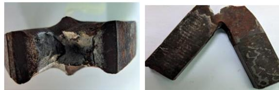
Gambar 3.13 patahan PWHT 850°C
