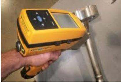
**Gambar 3.1. Positive Material Identification**
