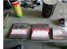
Gambar 4.2 hasil proses NDT liquid penentran
