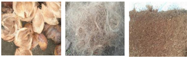
Figure 4.2 Materials and Products: a) Coir before decomposition, b) Coconut fiber after decomposition (Cocofiber), c) Cocoair powder (Cocopeat)
