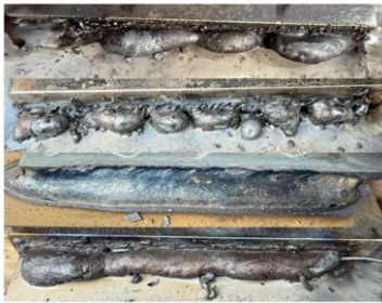
Fig. 1. Effect Of Poor Welding Parameter Selection [8]
