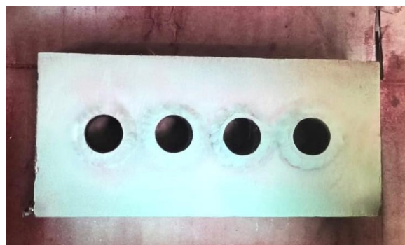
Fig. 6. Penetrant test result
