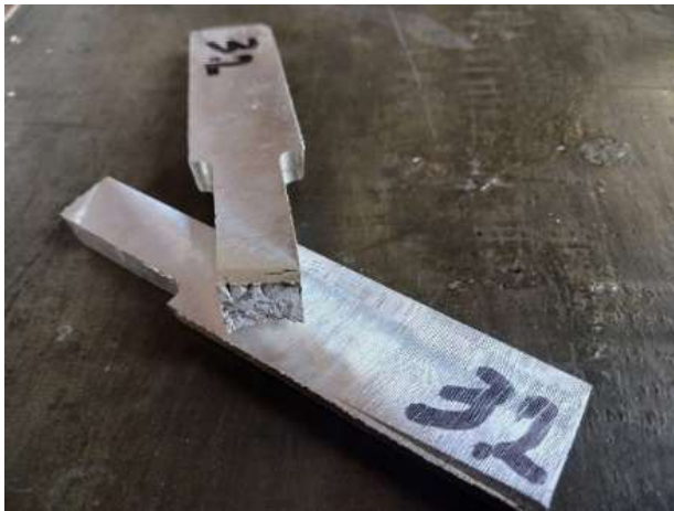
Fig. 7. The fracture of the tensile test
