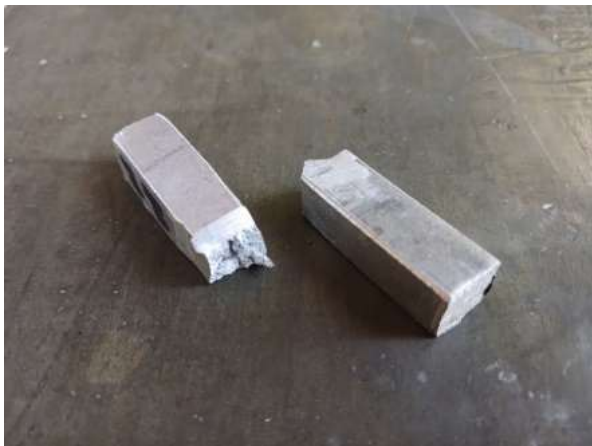
Fig. 4. The fracture of the impact test
