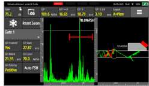
Fig. 8. Ultrasonic test results at 120 A current
