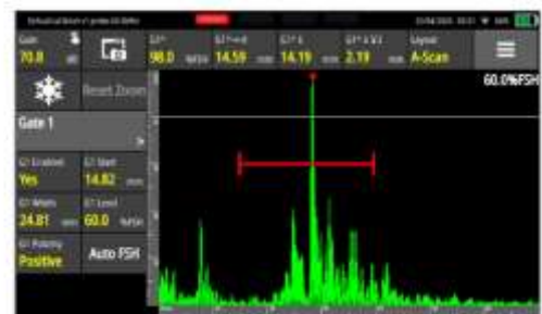
Fig. 3. Ultrasonic test results at 100 A current
