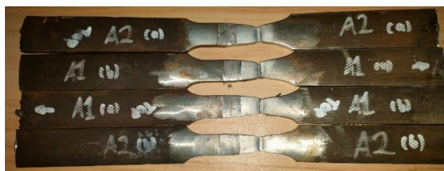
Fig. 5. Fracture location at tensile specimen
