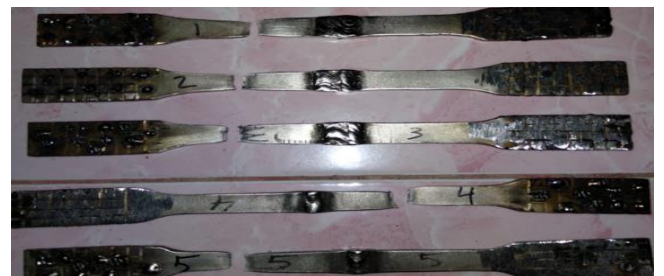
Fig. 6. Fracture results that occurred during the tensile test process for specimens with a protective gas flow of 8 L/min.
