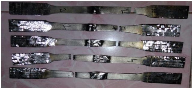
Fig. 7. Fracture after tensile test at a protective gas flow of 13 L/min.
