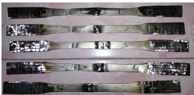
Fig. 8. Fracture after tensile test at a protective gas flow of 18 L/min.
