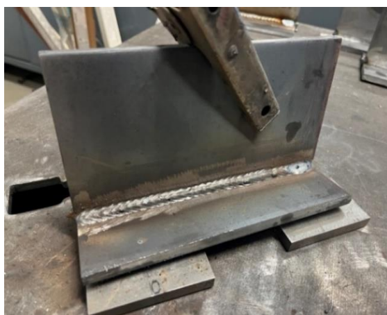
Fig. 12. Welded test specimen for bending experiment ready for initial inspection.
