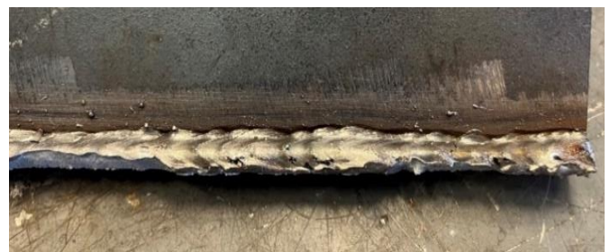
Fig. 16. Undercut on Failed B11 Test Specimen in fillet weld bending experiment.
