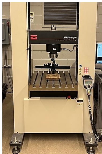
Fig. 13. MTS Systems (Eden Prairie, MN) Insight electromechanical press used in fillet weld bending experiment.
