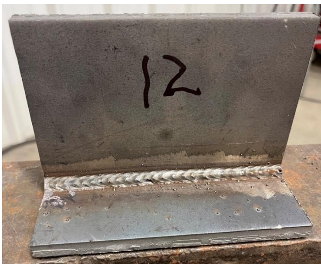
Fig. 20. B12 test specimen from the fillet weld bending experiment.
