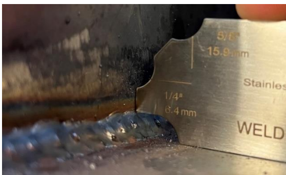
Fig. 8. Measuring fillet weld with manual fillet weld gauge.
