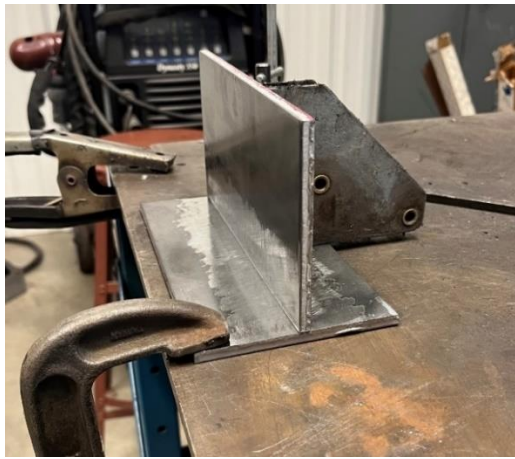
Fig. 7. Plate configuration for welding pieces into fillet weld bending experiment test sections.
