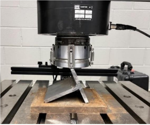
Fig. 15. Test specimen in MTS Systems (Eden Prairie, MN) Insight electromechanical press during fillet weld bending experiment.
