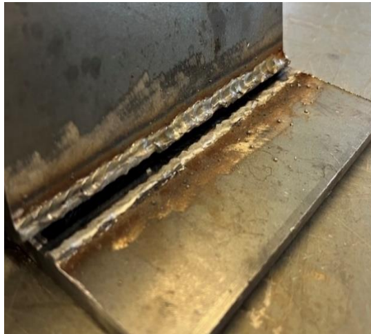
Fig. 17. Failed A1 Test Specimen through lack of fusion into bottom plate during fillet weld bending experiment.
