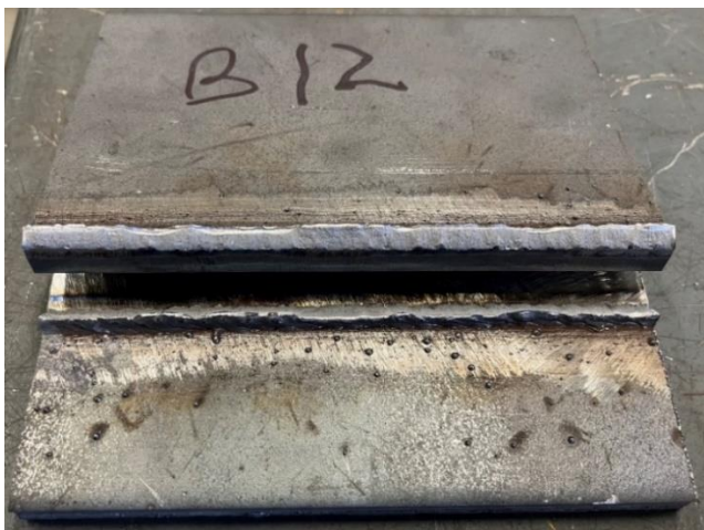
Fig. 21. Fracture down the center of the weld axis of the B12 test specimen from the fillet weld bending experiment.
