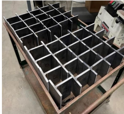
Fig. 10. Weld test specimens for bending experiment with Sample A on left and Sample B on right.
