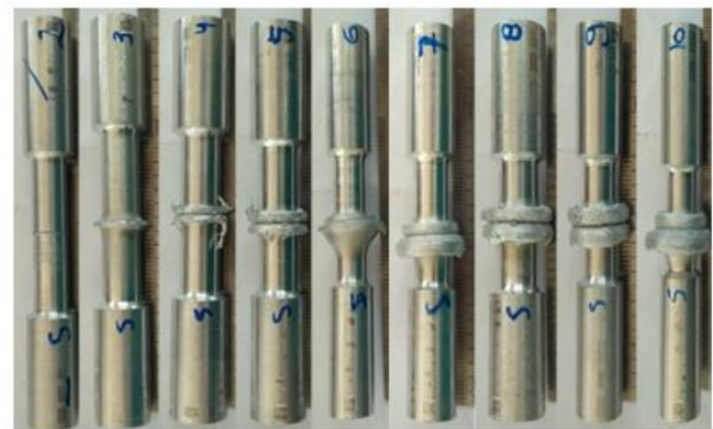
Fig. 4. Results of joining 6061 aluminum CDFW
