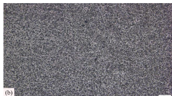
Gambar 12. Struktur Mikro weld metal : (a) cold bending , (b) hot bending .
