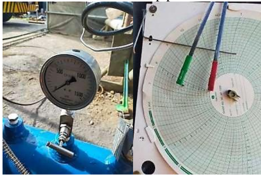
Fig. 15 Pressure 0 Psi and Chart Recorder 0 Psi
