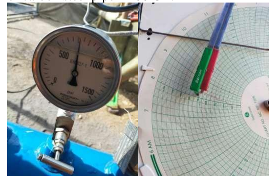
Fig. 18 Pressure 690 Psi Chart Recorder Pressure 690 Psi
