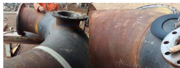
Fig. 3 A106 Gr. B Carbon Steel Pipe (U Tube Seal Deck shaped) cleaned of paint layer and cut [7]
