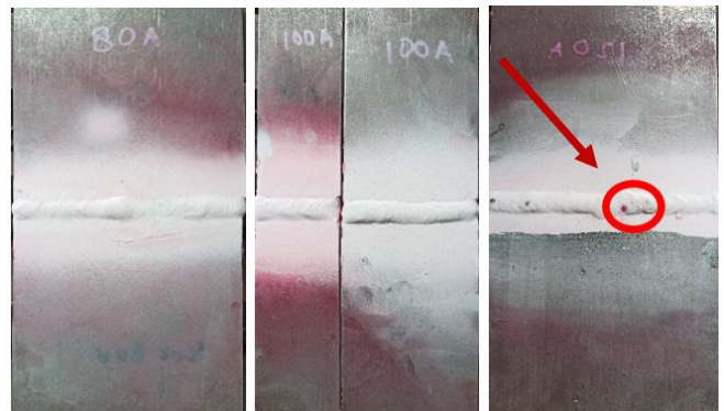
Fig. 6. Penetrant Test Results
